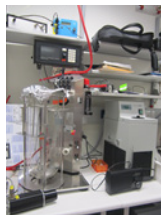
Left: Anaerobic, artificial rumen in the laboratory used to trickle-feed Pimelea to rumen fluid samples in pursuit of rumen bacteria that can breakdown the toxin.
